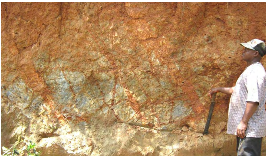
Figure 9.F: Road cut exposing Auriferous Quartz-carbonate Vein Stockwork in Saprolitic Quartz Diorite (Zone 2 - trench TKB005 granitoid zone)
